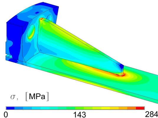
**Figure 5:** The distribution of the von Mises stress in the flange connection of the steel pipe line
