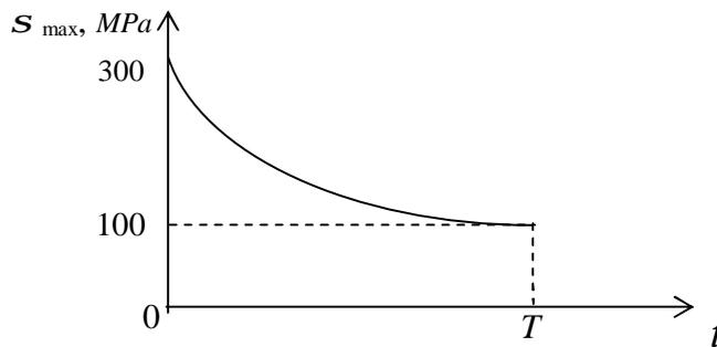
**Figure 4:** The relaxation of the yield stress in steel with time in the presence of hydrogen
