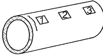
Figure 4: Scheme of probe position with respect to the crack in titanium tube.
