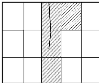
Figure 5: Map of hydrogen distribution in the plate. Thick shading – 2.0 ppm; sparsely shading – 1.7 ppm; in another parts – 1.2-1.3 ppm.
