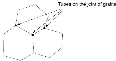
Figure 6: Scheme of the defect position on the joint grains
