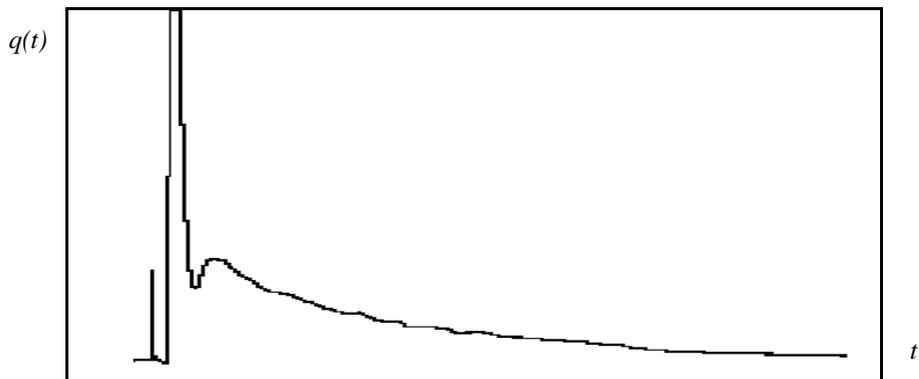
Figure 10: Experimental extraction curve for the titanium alloy PT-7M
