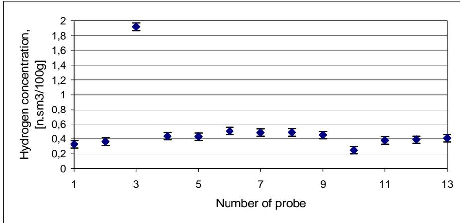
Figure 3: Results of analysis of hydrogen content in SSP of the alloy AMg-6
