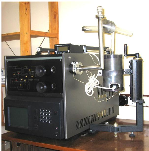
Figure 1. Hydrogen analyzer AV-1
