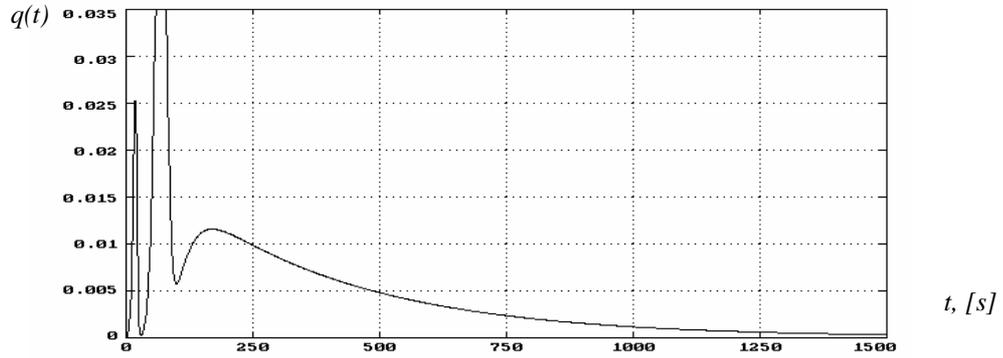
Figure 9: Calculated extraction curve with three maxima
