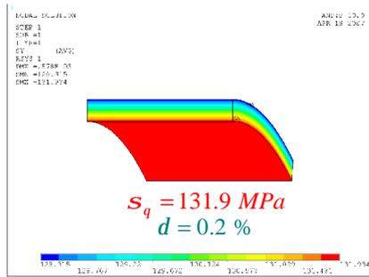
**Figure 7:** Tangent stress in the remote region of the pipe
