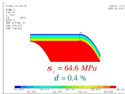
**Figure 8:** Axial stress in the remote region of the pipe
