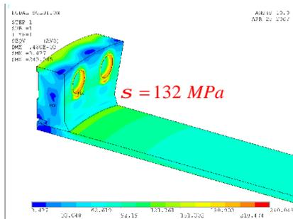
**Figure 15:** Stress in the pipe line before hydrogen saturation
