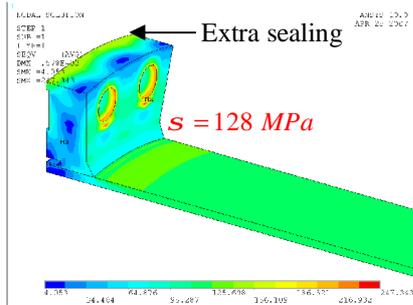
**Figure 13:** Stress in the pipe line before hydrogen saturation
