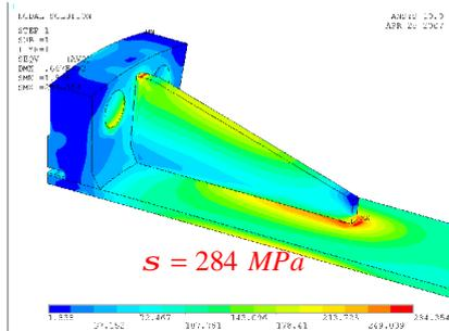
**Figure 9:** Stress in the pipe line before hydrogen saturation
