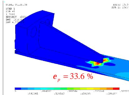
**Figure 10:** Plastic strain after hydrogen saturation
