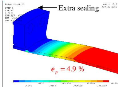
**Figure 14:** Plastic strain after hydrogen saturation
