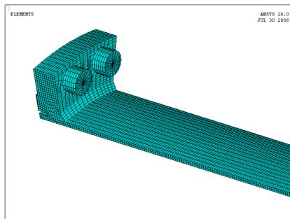
**Figure 6:** Finite element model of 20° sector
