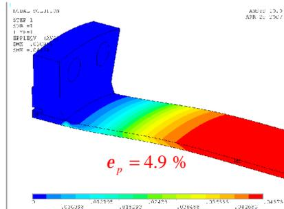
**Figure 12:** Plastic strain after hydrogen saturation
