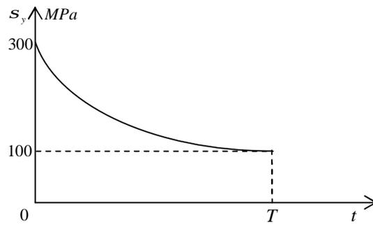
**Figure 4:** Yield strength decrease at hydrogen saturation
