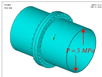
**Figure 5:** Flange connection of the pipe line
