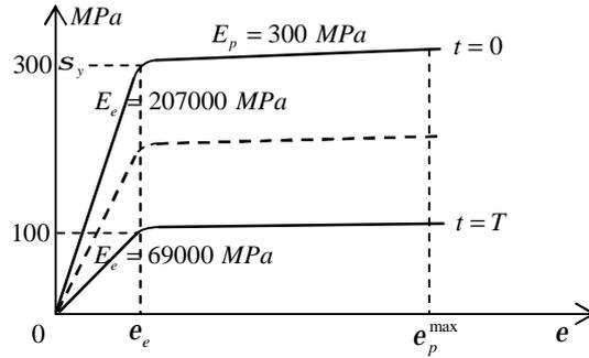
**Figure 3:** Steel stress strain curve
