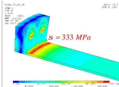
**Figure 11:** Stress in the pipe line before hydrogen saturation
