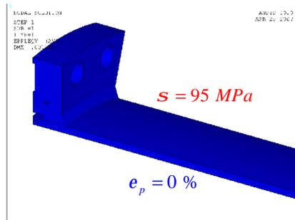
**Figure 16:** Plastic strain after hydrogen saturation
