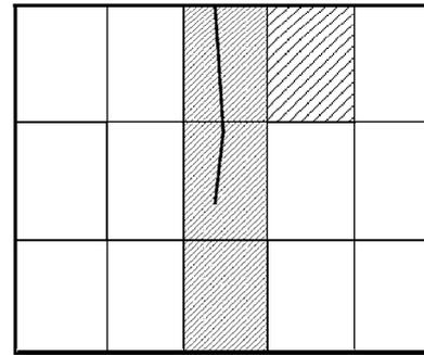
Figure 4: Map of hydrogen distribution in the plate. Thick shading – 2.0 ppm; sparsely shading – 1.7 ppm; in another parts – 1.2-1.3 ppm.
