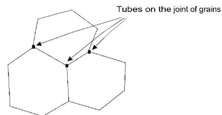
Figure 5: Scheme of the defect position on the joint grains
