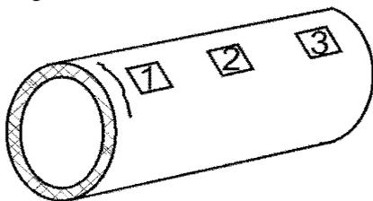
Figure 3: Scheme of probe position with respect to the crack in titanium tube.
