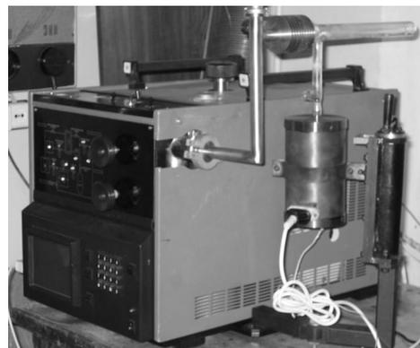
**Figure 1:** Hydrogen analyzer AV-1
