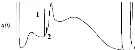
**Figure 9:** Experimental extraction curve for the aluminum alloy AD-31
