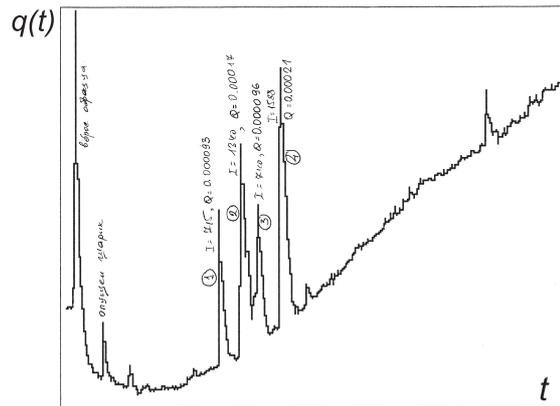
Figure 1: The part of the extraction curve for aluminum alloy D-16 with small peaks
