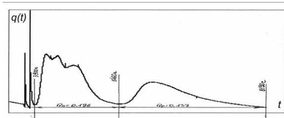
Figure 8: The extraction curve fore pure aluminum A8
