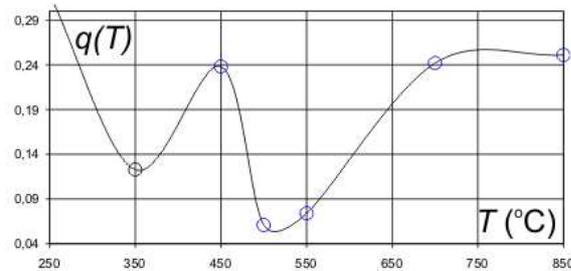
Figure 9: The extraction curve for nanocrystalline stainless steel
