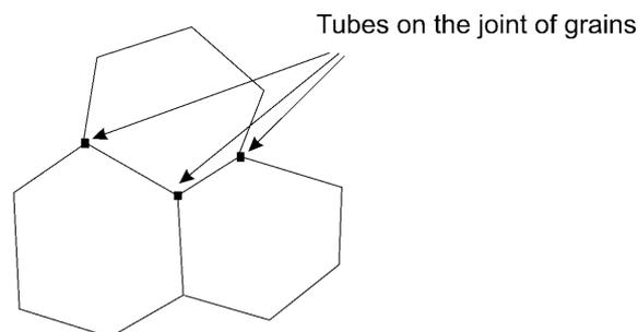
Figure 7: Scheme of the defect position on the joint grains
