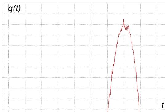
Figure 6: The fragment of the extraction curve - emission of hydrogen from sample of St 70 without zinc layer
