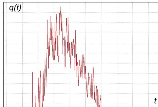
Figure 5: The fragment of the extraction curve - emission of hydrogen from sample of St 70 with zinc layer  $h=10 \mu\text{m}$
